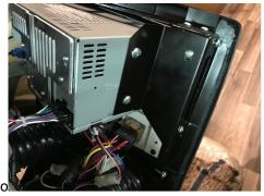
The Driver's Side mount would only have one screw holing a single din radio It may require an additional bracket to provide the needed stability
